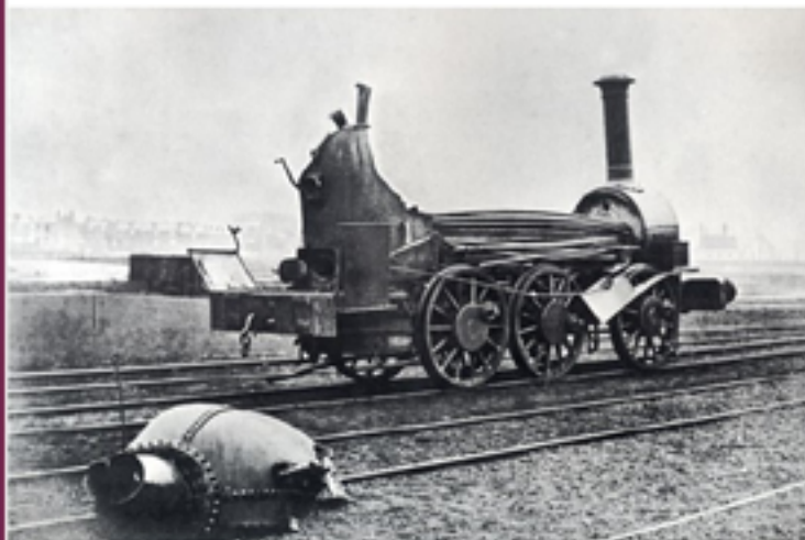
York Newcastle & Berwick Railway, Darlington, 2nd February 1850, three people died. Appears to be a Kitson long-boiler of around 1845 (note the staggered spokes), as supplied to the York and North Midland Railway.
