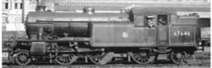
V1 had 190lbs boilers. V3 had 200lbs boilers
