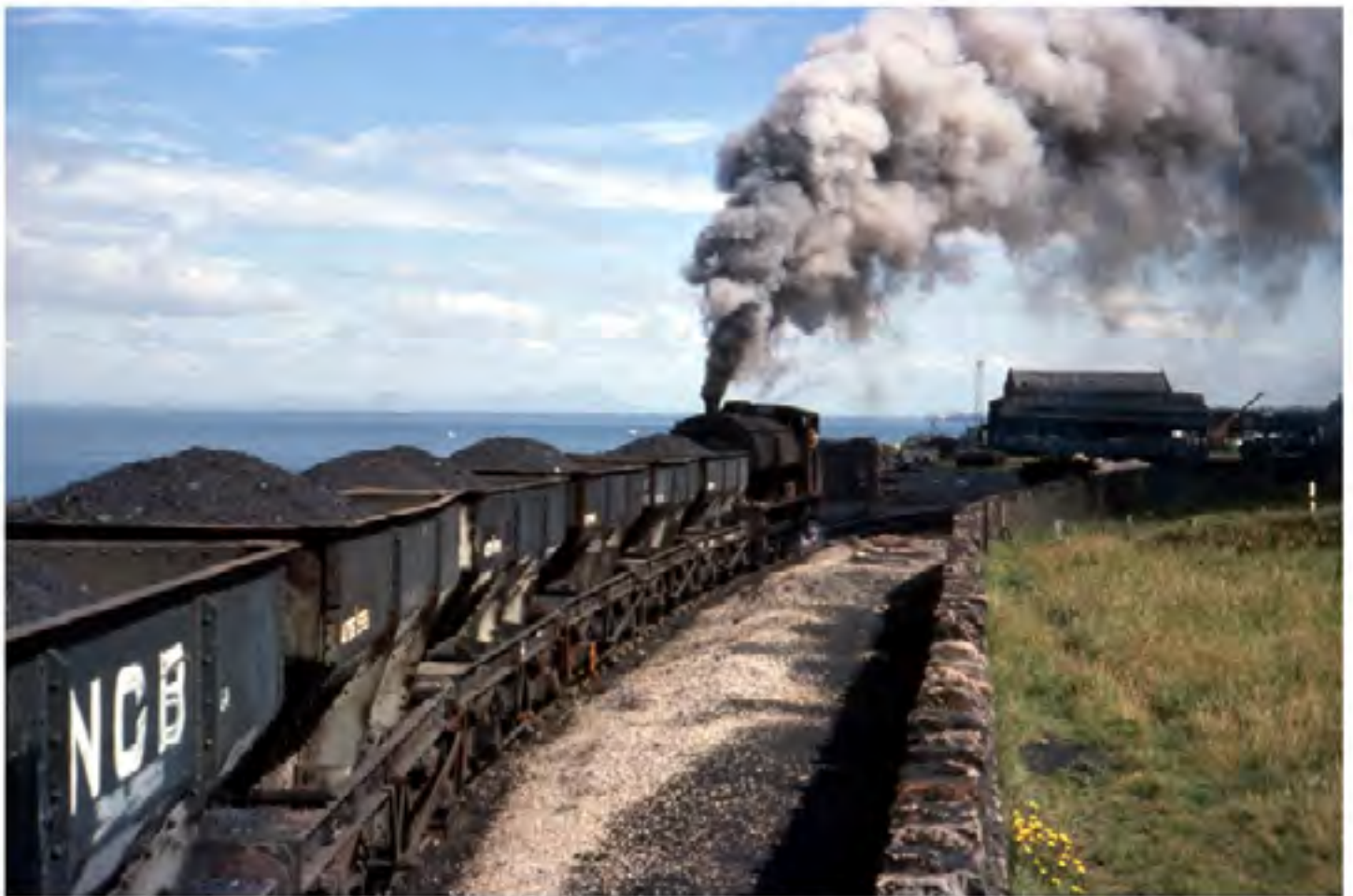
Haig Colliery, Whitehaven in June 1974 showing 0-6-0ST Austerity 'Respite' built by Hunslet in 1950
